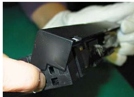
press and pull back anti-static guard - VHS
